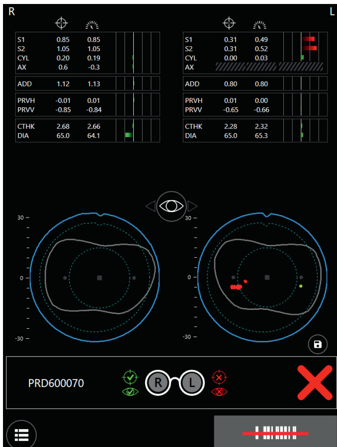
Fig. 3 : Full lens inspection. Metrology results displayed at the top, cosmetic inspection in the middle, and a summary of the decisions at the bottom. Blue represents the lens edge, grey indicates the cut lens edge, red marks rejecting defects, and green denotes non-rejecting defects.
